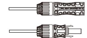
Figure 3.16 Connector with Cap nut Screwed on
