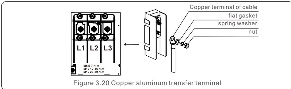
Figure 3.20 Copper aluminum transfer terminal
