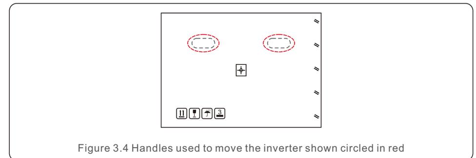
Figure 3.4 Handles used to move the inverter shown circled in red
