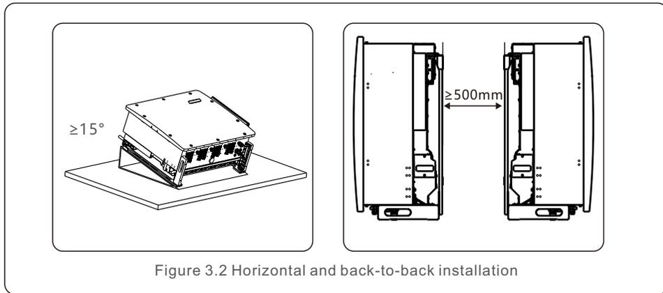
Figure 3.2 Horizontal and back-to-back installation
