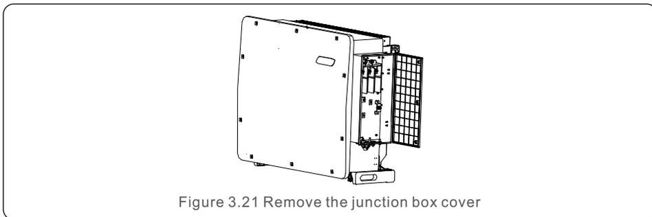
Figure 3.21 Remove the junction box cover
