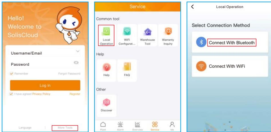
Step 2: Select the Bluetooth signal from the inverter. (Bluetooth Name: INV-Inverter SN)
