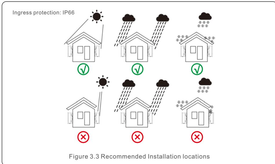
Figure 3.3 Recommended Installation locations
