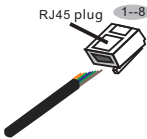
Figure 4.22 Strip the insulation layer and connect to RJ45 plug
