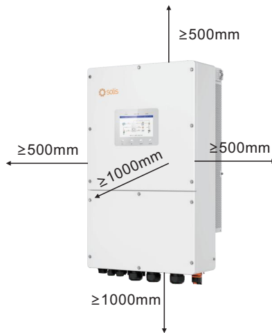
Figure 3.5 Inverter Mounting Clearances
