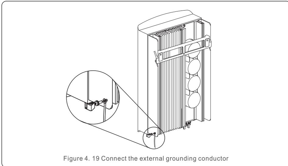
Figure 4.19 Connect the external grounding conductor
