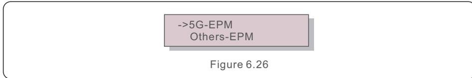
5G-EPM Failsafe Option should be turned ON when 5G series EPM device is used
