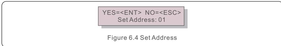
Press the UP/DOWN keys to set the address. Press the ENTER key to save the settings. Press the ESC key to cancel the change and return to the previous menu.
