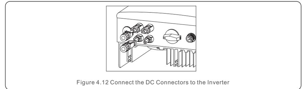
Figure 4.12 Connect the DC Connectors to the Inverter
