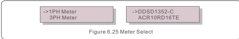
For Solis single phase inverters, please select "1PH Meter" and then select the corresponding meter model.
