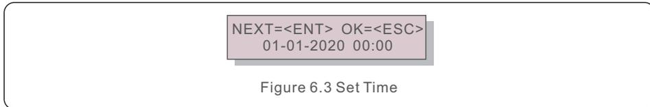
Press the UP/DOWN keys to set time and data. Press the ENTER key to move from one digit to the next (from left to right). Press the ESC key to save the settings and return to the previous menu.
