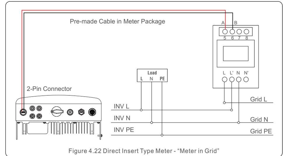
Figure 4.22 Direct Insert Type Meter - "Meter in Grid"
