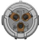
Figure 4.4 AC Grid Terminal Connector Inside
