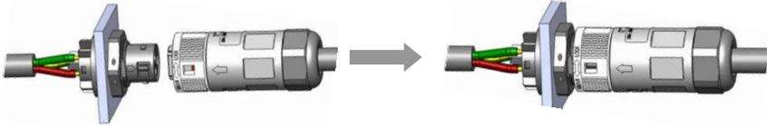
Figure 4.9 Connect the AC Connector to the Inverter
