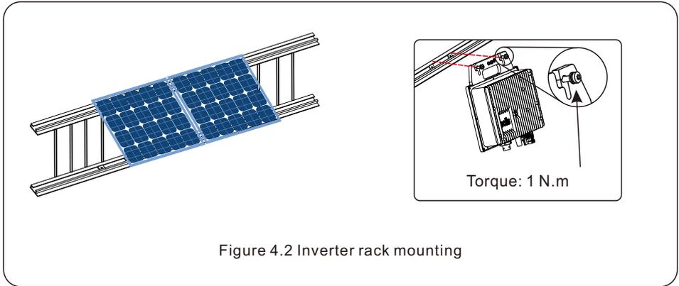
Figure 4.2 Inverter rack mounting
