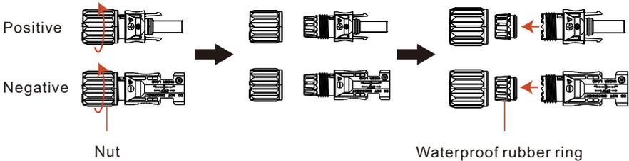
Figure 4.11 Remove the cover of the terminal connector
