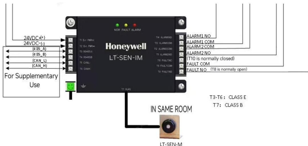
Figure 7-4 Flammable gas detector wiring diagram
