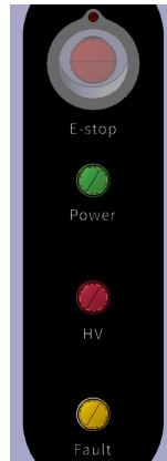
Figure 6-5 System operation. Indicator on cabinet door
