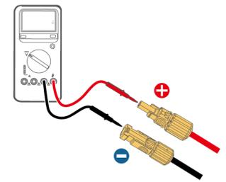
**EN** Recommended connections of DC input terminals
